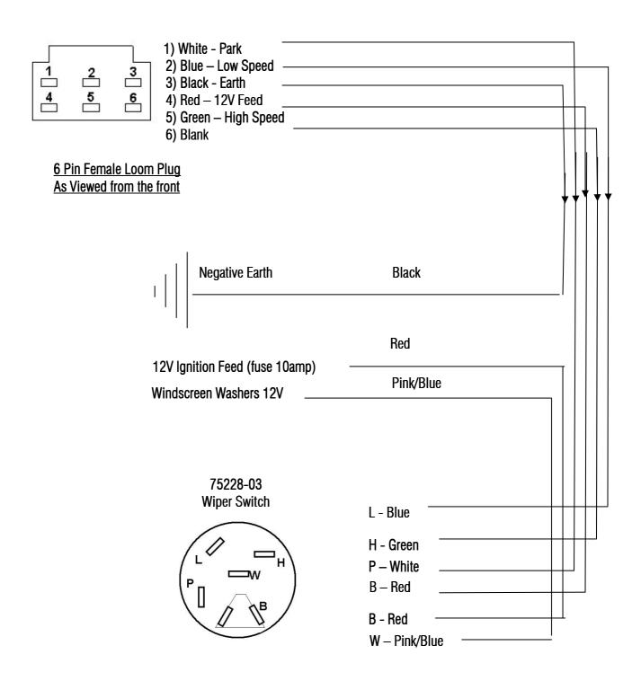
Wiper switch system is 12V Positive Feed
